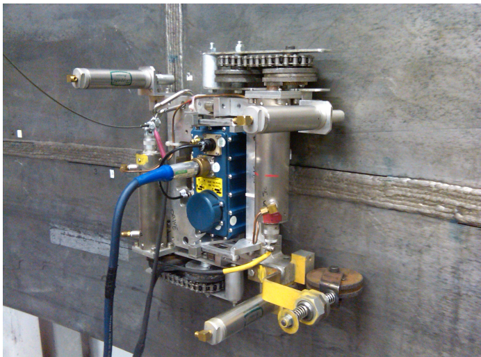
ACFM Crawler and Probe on Test Plate
